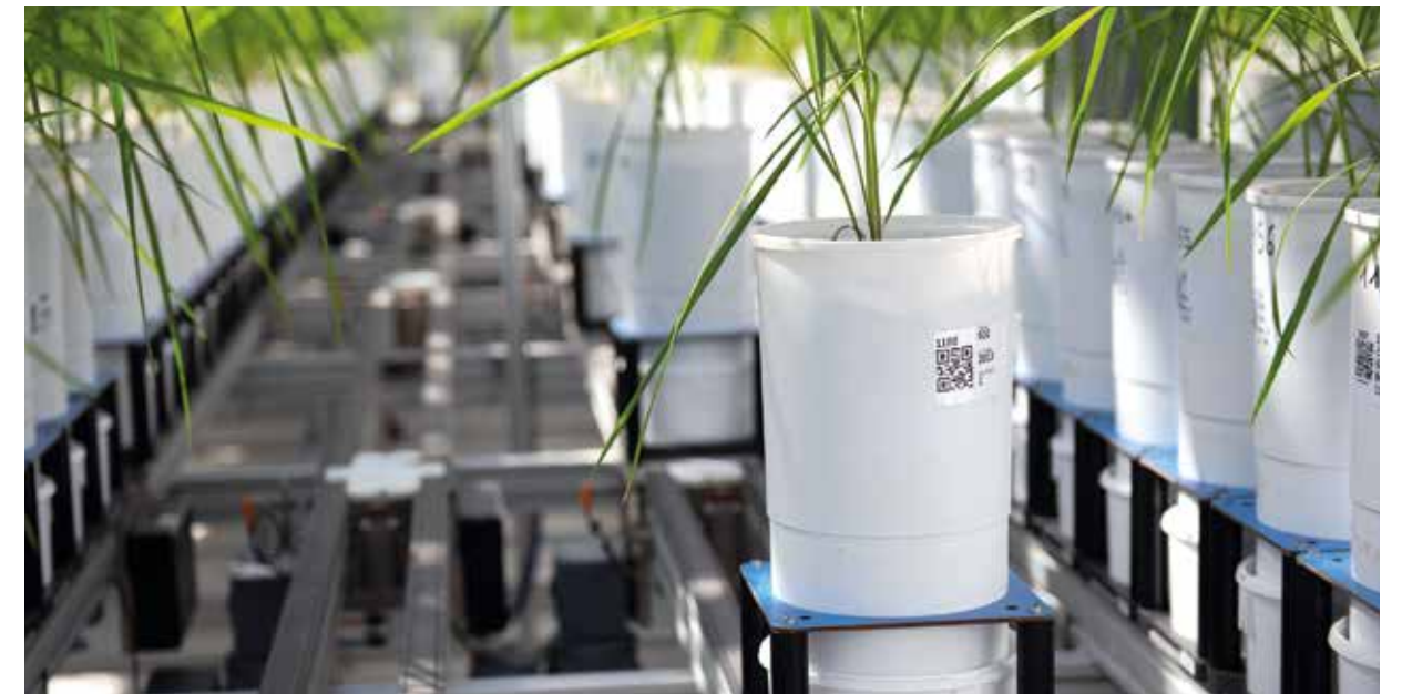
High-throughput phenotyping platform at the Joint Research Unit for the Ecophysiology of Plants under Environmental Stress (LEPSE) in Montpellier. The laboratory analyses and models the genetic variability underlying plant responses to extreme environmental conditions, notably drought and high temperatures. © INRAE, C. Maitre
