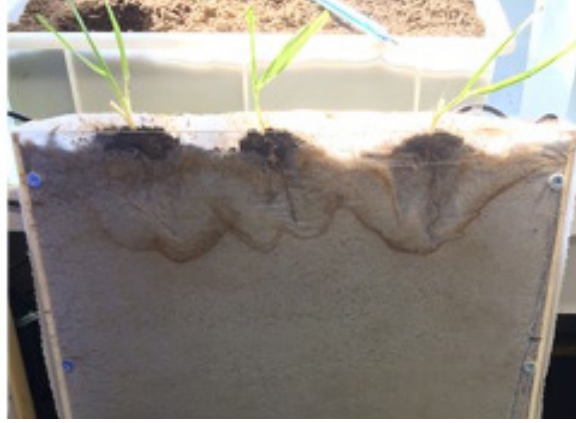
©Magali Nuixé- Front view of a rhizotron containing three cocksfoot ( Dactylis glomerata ) plants separated from the ground by the cloth at the time of its installation.
