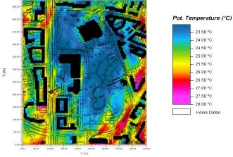
Figure 4 - Air temperature (° C) in and around an urban park in Essen (Germany); (Lahme and Bruse, 2003)
